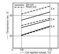
4-(2) Influence of adjacent mounting Tested sample: DS2Y-S-DC12V, 10 pcs. Ambient temperature: 20°C 68°F
